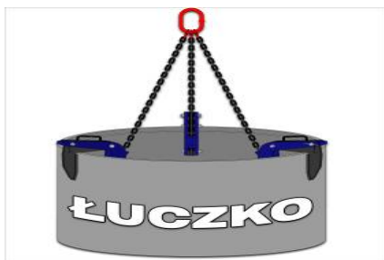
ZŁ 3C gripping range 50-180mm Permissible work load 3000 kg weight 55kg
